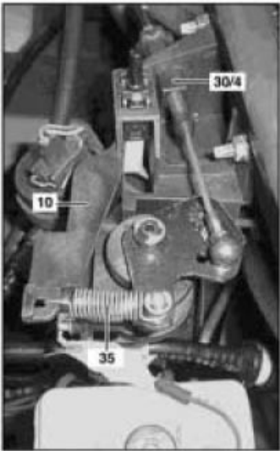
Fig. 19: Identifying Throttle Control Components - Shown On Engine 112.942 In Model 163.154
